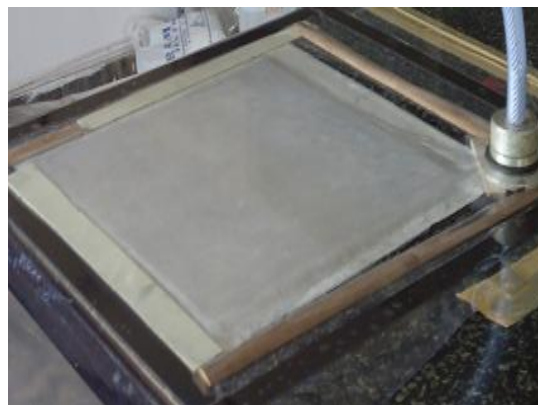
Figure 2: Vacuum bag process
